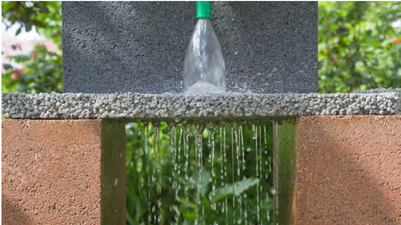
Permeable paving reduces stormwater runoff and recharges groundwater
